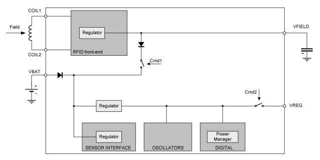
The power management mode is defined by the switches Cmd1 and Cmd2 and is configurable through the EEPROM and EE-Latch.
