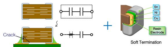
> Serial construction of inner electrode prevents sudden insulation breakdown after flex crack formation.
