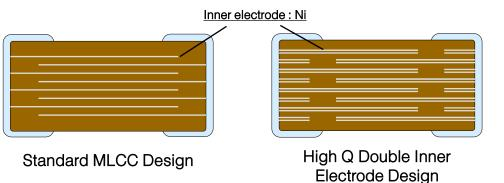
➤ ESR of the High Q capacitor can be 30%-50% lower than ESR of a STD MLCC due to the double inner electrode design.
