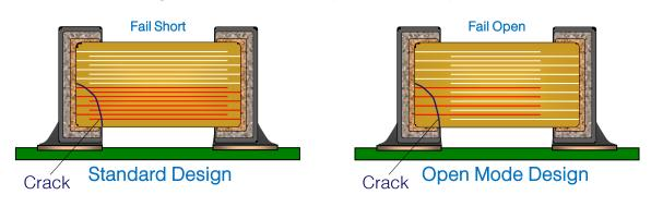
> Open Mode capacitor is designed with wider gap between the terminal and the internal electrodes to help reduce the risk of short circuit in the event of capacitor cracking due to mechanical stress such as board bending.
