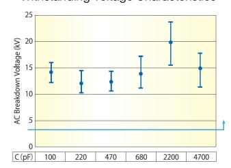
Withstanding Voltage: 4kVAC/60s, High breakdown voltage level
