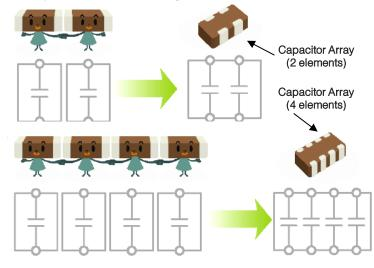
Array Capacitor combines multiple capacitor into a single chip. They are effective in reducing placement time and cost.
