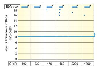
High impulse voltage characteristics based on International Standard IEC60384-14; Impulse test (8kV)
