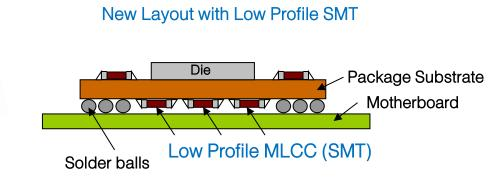
By using low profile MLCC, it is possible to mount MLCC between BGA and motherboard and save space on PBC.
