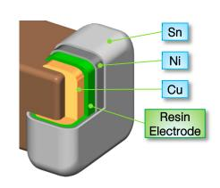
> Soft termination is available for 2in1 Array capacitor. A resin electrode layer between the copper base and the nickel plating of the terminal electrode absorbs bending stress from the board and suppresses the forming of solder cracks.
