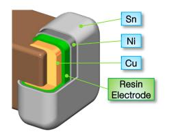
> A resin electrode layer between the copper base and the nickel plating of the terminal electrode absorbs bending stress from the board and suppresses the forming of solder cracks.
