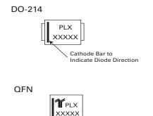
Cathode Bar to Indicate Diode Direction
