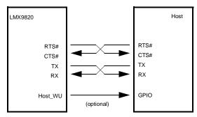
Figure 16. UART NULL modem connection
