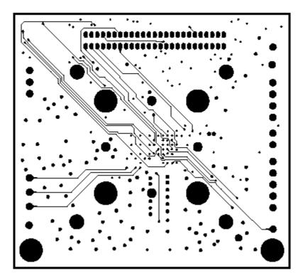
Figure 24. Signal Plane - Layer 3
