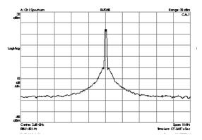
Figure 6. Synthesizer Phase Noise
