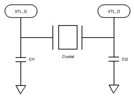
Figure 10. LMX9820 Crystal Recommended Circuit
