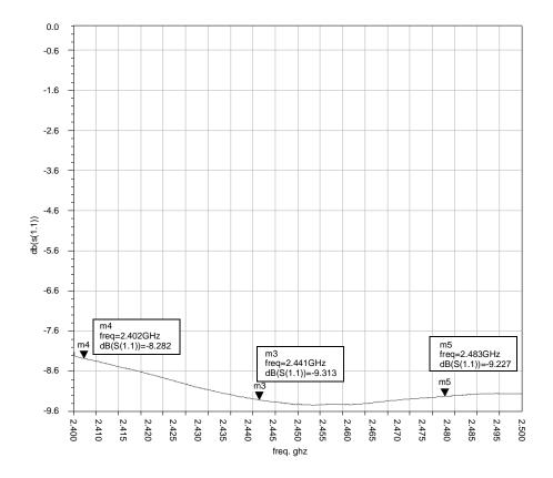
Figure 9. Transceiver Return Loss
