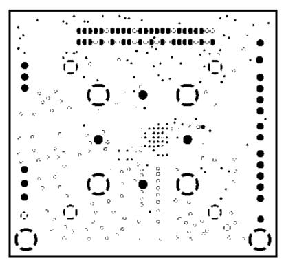
Figure 23. Solid Ground Plane - Layer 2
