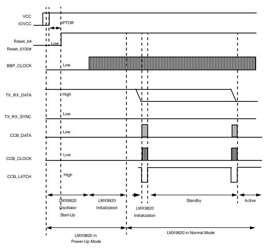
Figure 14. LMX9820 System Power-Up Sequence Timing
