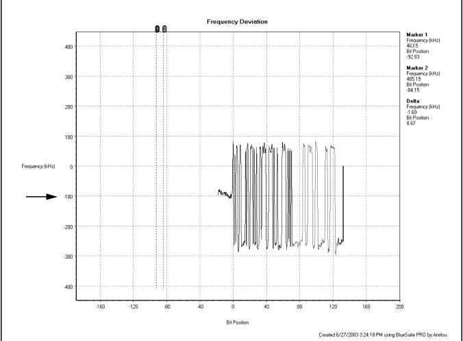
Figure 12. Frequency Offset with 10 pF // 10 pF Capacitors
