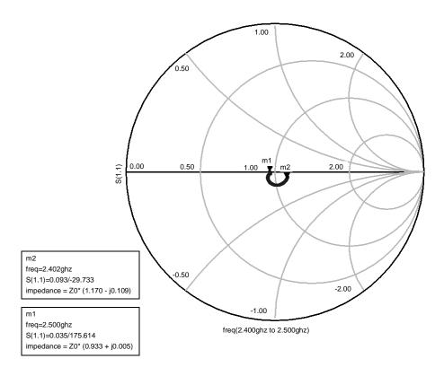
Figure 8. TX and RX Pin 50 $\Omega$  Impedance Characteristics
