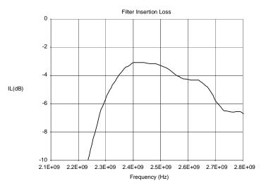
Figure 7. Front-End Bandpass Filter Response
