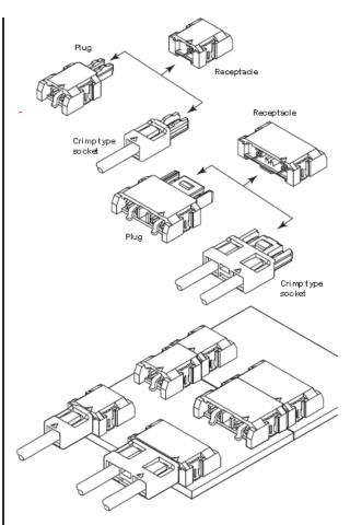
Designed for LED light bar applications, the low profile of the connector does not interfere with the *luminescence* angle of LED dies. The LEB Series provides both board-to-board and wire-to-board capabilities. The board-to-board plug and receptacle connectors allows continuous connection of LED light bars
