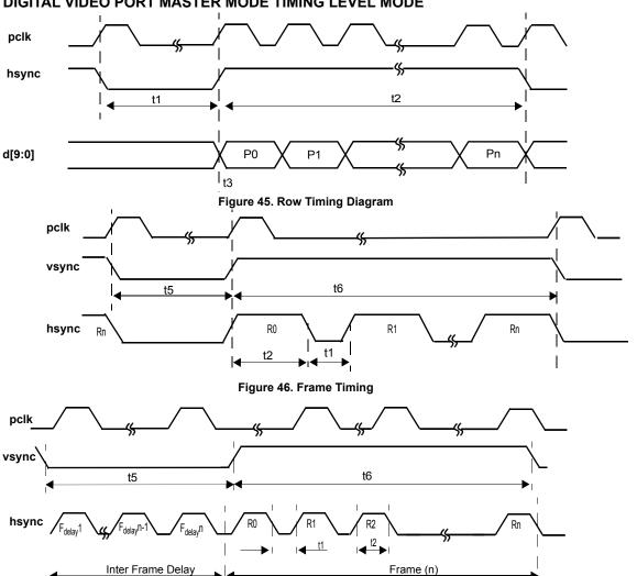
Figure 47. Frame Delay Timing (With Inter Frame Delay).
