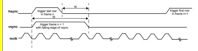
Figure 52. Slave Mode d[9:0], hsync & vsync to pclk Timing
