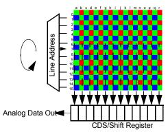
Figure 7. CMOS APS Row and Column addressing scheme
