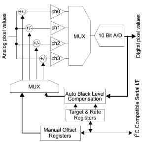
Figure 8. Analog Signal Conditioning & Conversion to Digital
