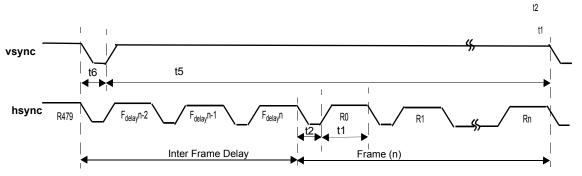
Figure 50. Frame Delay Timing (With Inter Frame Delay).
