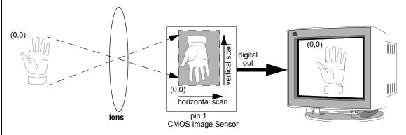
Figure 4. Scan directions and position of origin in imaging system
