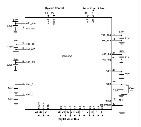
Figure 3. Typical Application Diagram
