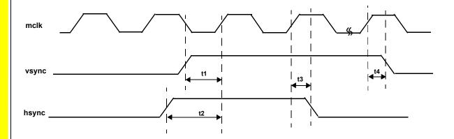
Figure 54. Set up and Hold Times for Slave Mode
