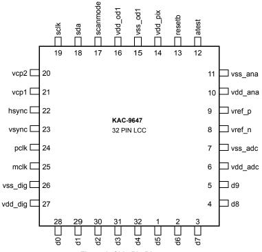
Figure 2. Chip Pin Diagram
