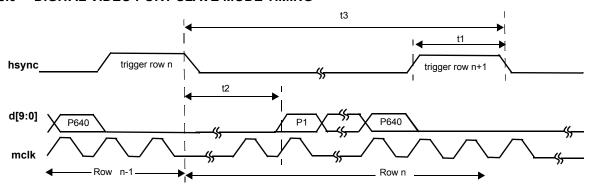
Figure 51. Slave Mode Row Trigger and Readout Timing
