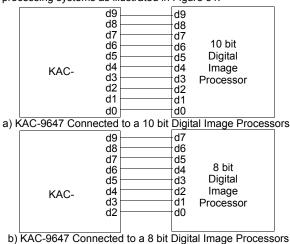
Figure 31. Example of connection to 10/8 bit systems
