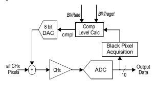
Figure 22: Digital Black Level & Offset Adjustment Loop
