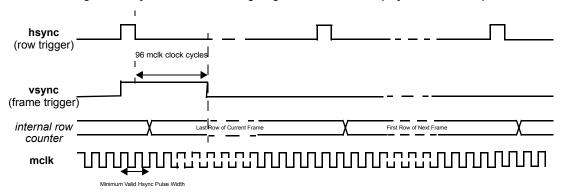
Figure 44. vsync slave mode timing diagram.
