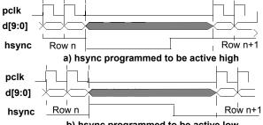
b) hsync programmed to be active low Figure 36. hsync in Pulse Mode
