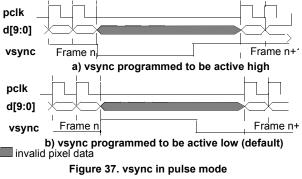
By default the first pixel data at the beginning of each frame is placed on the digital video bus as soon as **vsync** is activated. Furthermore, **vsync** is de-activated upon the placement of the last pixel of the current frame on the digital video bus. It is possible to shift the start and end edges of the **vsync** signal by programming the *VsyncStart* parameter of the DVBUSCONFIG0 register and the *VsyncEnd* parameter of the HYSNCADJUST register.
