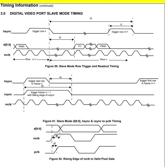
The following specifications are from simulation. For the minimum value the conditions are all supply pins = +3.0V &  $C_L$  = 5pF and 0C while the maximum value conditions are all supply pins = 3.6V &  $C_L$  = 25pF.
