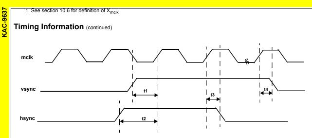
Figure 53. Set up and Hold Times for Slave Mode
