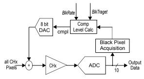
Figure 21: Digital Black Level & Offset Adjustment Loop
