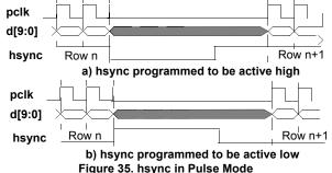
By default the first pixel data at the beginning of each row is placed on the digital video bus as soon as **hsync** is activated. Furthermore, **hsync** is de-activated upon the placement of the last pixel of the current row on the digital video bus the digital video bus. It is possible to shift the start and end edges of the **hsync** signal by programming the *HsyncStart* parameter of the DVBUSCONFIG0 register and the *HsyncEnd* parameter of the HYSNCADJUST register.
