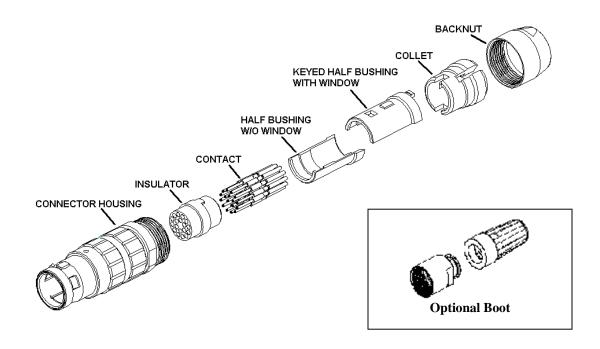
1. Determine what size cable you will be using. Then select the proper collet number for that cable.
