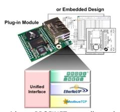
incorporating a *RapID Platform Network Interface* will operate problem-free with any PROFINET controller and will never disconnect from the network.
