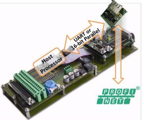
the Host to the UART or 16-bit Parallel interface. The Ethernet physical interface is ready to plug into the network. Software for the module is provided as firmware that is resident on the flash.
