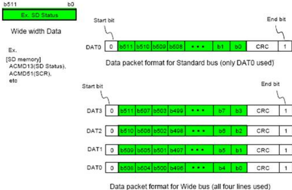
Figure 6-7: Data packet format - Wide width data
