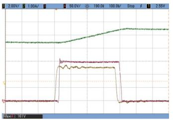
Figure 4: Waveforms for V<sub>IN</sub> = 150 V to 5 V/5 A (100kHz) Buck converter CH1: V<sub>PMM</sub> Input voltage – CH2: (I<sub>OUT</sub>) Switch node current – CH4: (V<sub>OUT</sub>) Switch node voltage
