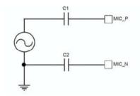
Single-ended Microphone Input (C1 and C2 should be 15nF).
