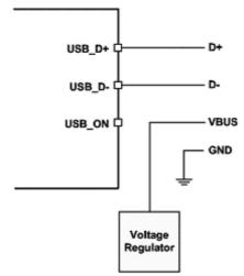
Connections to F2M03 for Bus-Powered Mode
