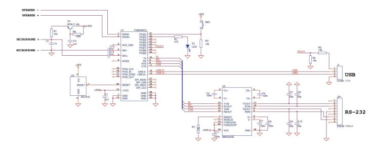
All capacitors in the schematic above are ceramic and must be mounted as close as possible to its respectively IC.
