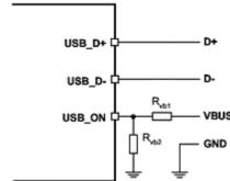
Connections to F2M03 for Self-Powered Mode
