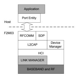
Embedded Two-Processor Architecture
