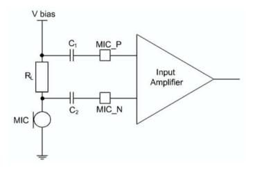
The input impedance at MIC\_N and MIC\_P is typically  $20k\Omega$ . C1 and C2 should be 47nF. R<sub>L</sub> sets the microphone load impedance and is normally between 1 and  $2k\Omega$ . V bias should be chosen to suit the microphone and have sufficient low *noise*. *It may be* obtained by filtering the *output of a PIO* line. (Subject to firmware support, consult available application notes and datasheets or contact free2move)
