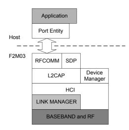
RFCOMM, (Embedded Two-Processor Architecture)
