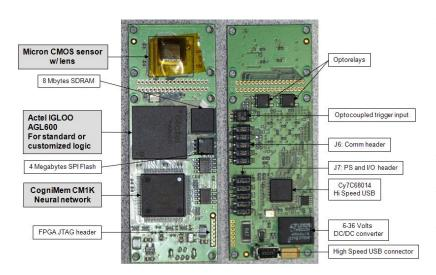
Access to all the components of the board is made via a simple Register Transfer Level (RTL) protocol. The CogniMem chip be used can independently from the recognition engine, to learn and recognize vector data transmitted from a host. FPGA programmers can implement their own feature extraction, results conditioning, and transmission to run on the board as an embedded platform.
