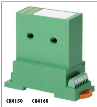
Two Element - 0.26" Window 0.5 to 30 AAC Input Range
