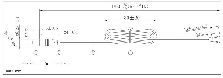
tolerance X: ±0.5 mm .X: ±0.3 mm .XX: ±0.05 mm applicable unless otherwise indicated in specification or on drawings Tensility International Corporation reserves the right to substitute
