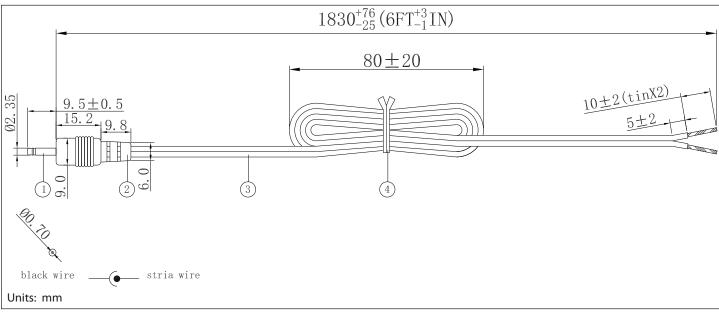
**tolerance** X: ±0.5 mm .X: ±0.3 mm .XX: ±0.05 mm applicable unless otherwise indicated in specification or on drawings Tensility International Corporation reserves the right to substitute parts which are functionally equivalent to the ones specified.
