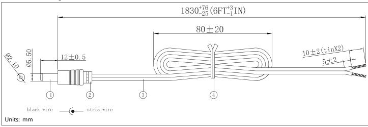
**tolerance** X: ±0.5 mm .X: ±0.3 mm .XX: ±0.05 mm applicable unless otherwise indicated in specification or on drawings Tensility International Corporation reserves the right to substitute parts which are functionally equivalent to the ones specified.
