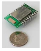
*Note:* SPI is for BlueRadios internal use only. Part is not 5Vdc tolerant. Reset is active **low**; pulse >5msec. PIO Sink Current is 4mA max. Unused pins can float accept for PIO(4), tie to ground if not used or disable via software.
