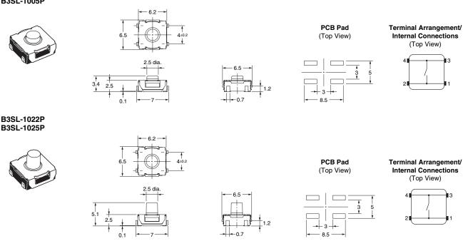
Note: Unless otherwise specified, a tolerance of ±0.4 mm applies to all dimensions.
