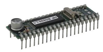
Using the VR Stamp<sup>™</sup> Toolkit, application programs can be downloaded into the VR Stamp. The VR Stamp can then be removed from the Module Programmer Board and plugged directly into the final product. In-circuit reprogramming is also supported.
