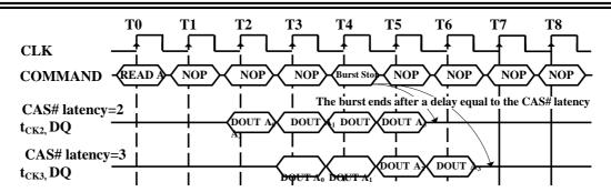
Figure 16. Termination of a Burst Read Operation (Burst Length > 4, CAS# Latency = 2, 3)
