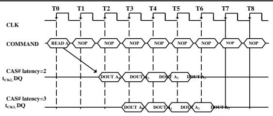
Figure 4. Burst Read Operation (Burst Length = 4, CAS# Latency = 2, 3)
