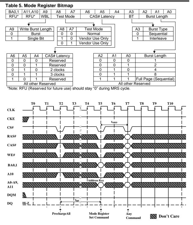
Figure 15. Mode Register Set Cycle
