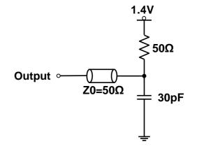
Figure 18.1 LVTTL D.C. Test Load (A)
