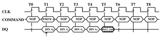
The first data element and the write are registered on the same clock edge
