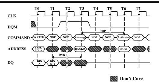
**Note:** The LDQM/UDQM can remain low in this example if the length of the write burst is 1 or 2.
