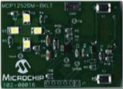
Demonstrates the use of a charge pump device in an LED application and acts as a platform to evaluate the MCP1252 device in general. Light intensity is controlled uniformly through the use of ballast resistors. A PIC10F206 MCU
