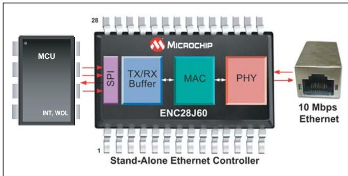
Microchip addresses the growing demand for a small and low-cost embedded Ethernet solution by offering the following:
