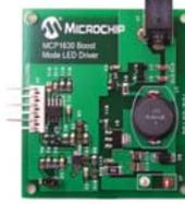
This demo board is a step-up, switch-mode, DC-DC converter used for power LED applications. The demo board provides a 350 mA or 700 mA constant current source with a jumper selection. The input operating voltage range is 9-16 VDC and the board can supply up to 30W to a string of power LEDs.
