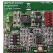
This board provides a SEPIC DC-DC converter for power LED and battery charging applications. The input voltage range is 3.5-16 VDC and the maximum power output is 8.5W.
