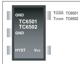
Low cost temperature sensing devices such as the TC6501 and TC6502 (offered in SOT-23 packages) can be conveniently placed near power LED(s) to obtain a more accurate temperature monitoring and provide a logic output fault signal.
