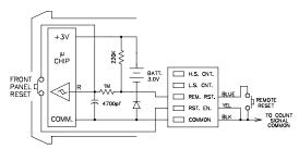
Connecting the "RST. EN." (Reset Enable) Input to Common activates the front panel Reset button. When the front panel Reset button is to be deactivated, remove the yellow wire from the "RST. EN." Input.
