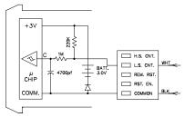
Pulling the "L.S. CNT." Input to Common with a mechanical or solid-state switch increments the counter. The low pass filter (*Imeg resistor and 4700 pf cap*) used with a Schmidt trigger circuit debounces mechanical switch signals. The switch load is  $14~\mu A$  (*max. voltage drop 0.5 V*) when ON. OFF-state leakage current must be less than  $2~\mu A$ .
