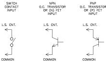
silver alloy relay contacts with wiping action are usually satisfactory for generating count input signals. Motor starter contacts, tungsten contacts, and brush-type contacts should **NOT** be used.
