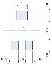
Note) The zero point is the center of mounting.
